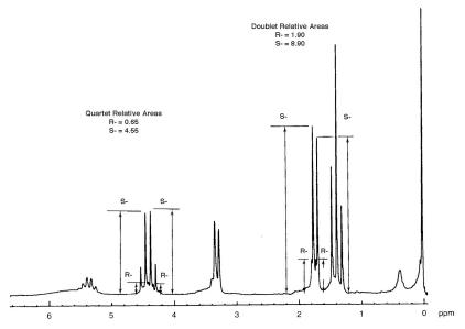
NMR of the enantiomeric excess product, plus chiral shift reagent: Method #3, Sodium Borohydride / Tartaric Acid Chiral shift reagent = Tris[3-(heptafluoropropylhydroxymethylene)-(+)-camphorato] europium III
