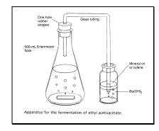
Add 100 mL of tap water, 30 g of sucrose, and about  $\sim$ 3.5 g (one package) of dry baker's yeast to the flask. Add these materials, while stirring, in the order indicated. Attach the trap to the fermentation flask. Stir this mixture for about 1 hour, preferably in a warm location. Add 4.0 grams of ethyl acetoacetate and stir the fermenting mixture vigorously at room temperature. Set aside and let stand until the next laboratory period.
