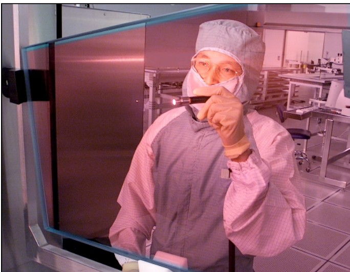
NIF laser glass under inspection prior to precision cleaning in the Optics Processing Development Laboratory.
