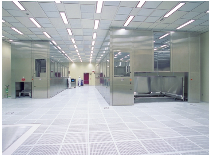
Automated equipment for precision cleaning of the large mechanical assemblies in the Optics Assembly Building.
