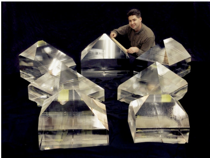
Large rapid growth KDP crystals for NIF. Approximately 35% of the NIF KDP crystal plates can be yielded from these boules.
